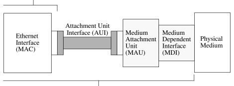
DTE With Internal MAU, AUI Not Exposed
